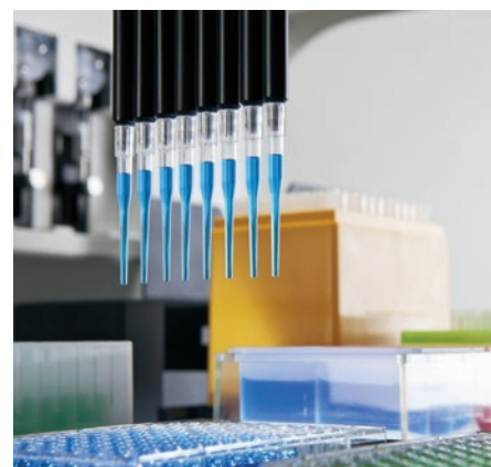
Figure 1. Biomek Span-8 pod with P250 (i-Series* 230 µL) wide bore pipette tips.
